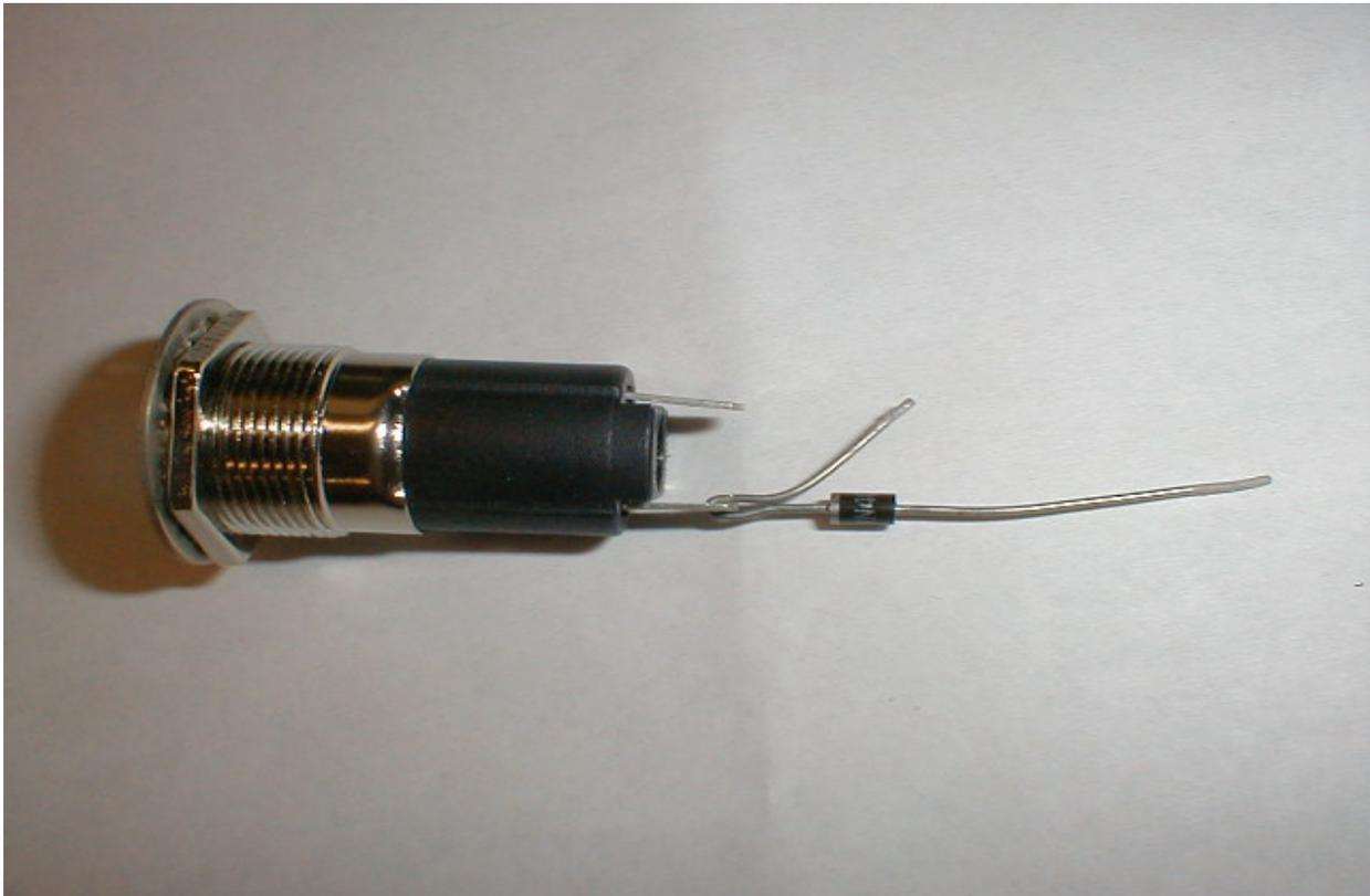
Trim the Diode so that it looks like this. You can use heat shrink tubing when you attach the wire to insulate the connection.
