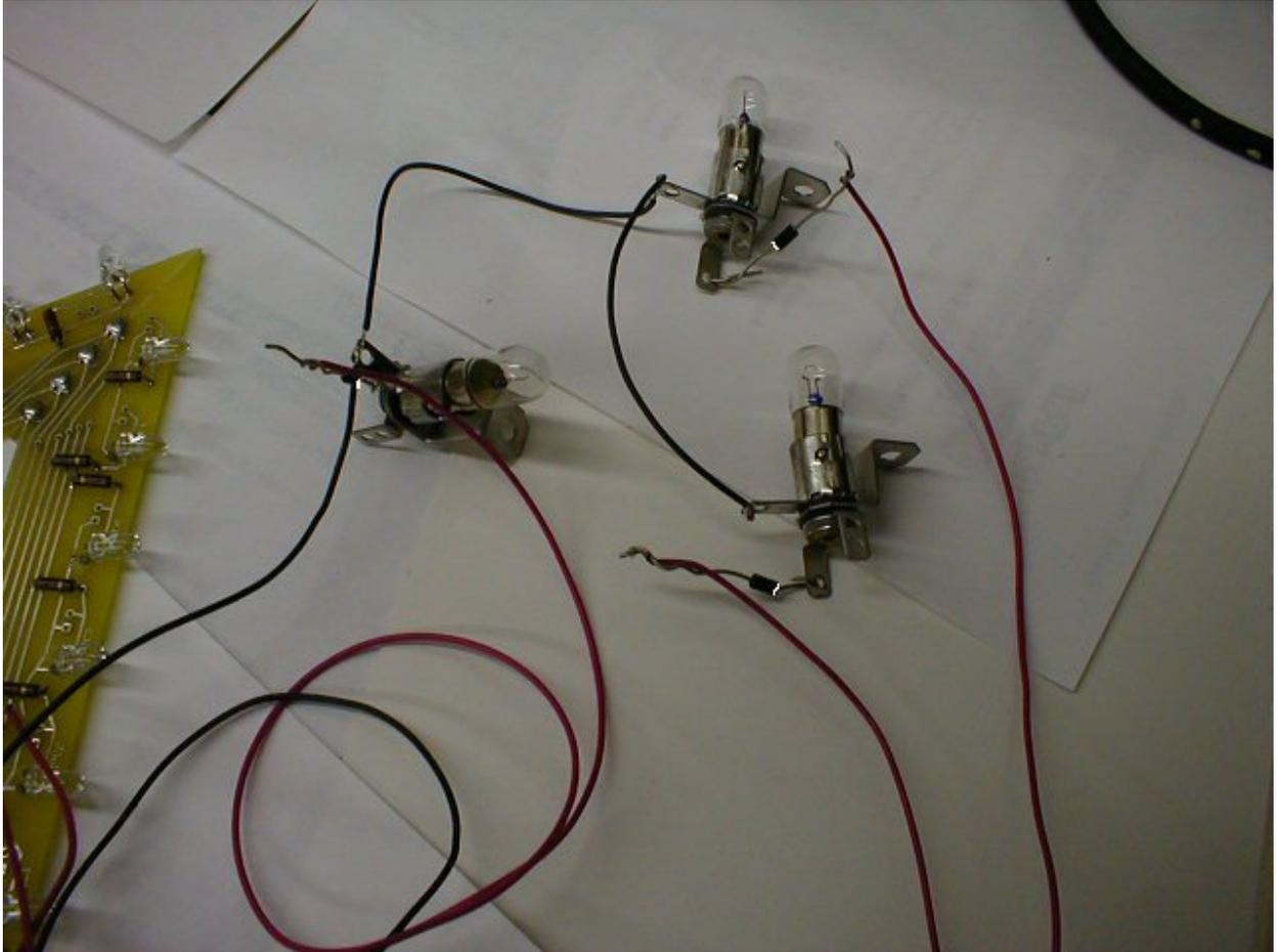
**Note:** The bulbs need to be 6VDC. The controller supply voltage can be between 12 and 18 volts DC, it will reduce this voltage for the lamps.
